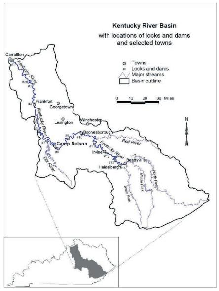
Figure 3. The location of the 14 locks and dams in the Kentucky River Basin, and key geographic sites mentioned in the text.
